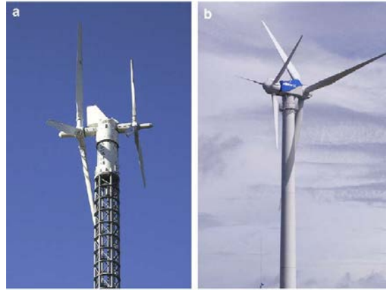
Figure 2 Double rotor wind turbine
